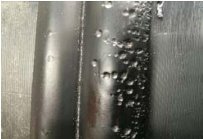
**Figure 3.** Example of a butt weld of black PE pipe affected by moisture at the jointing surface.
